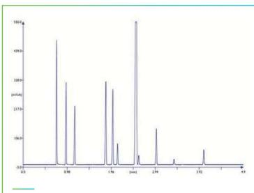
FIGURE 1: Gas chromatogram: Separation of residual solvents headspace GC using Avantor® Hichrom HI-VOC 2 FAST columns
